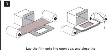
Lay the film onto the open box, and close the frame over the top.
