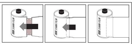
Light-safety is created by sandwiching the film between two layers of cardboard, and inserting those layers into the already light safe film canister. Carefully slide both tabs into the film canister, taking care to push the canister snugly against the frame.
